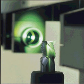
Non-contact measurement of tool cutting edges.
