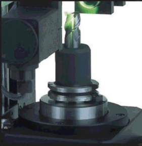
Precisely supported fixture spindle. 90°index (optional).
